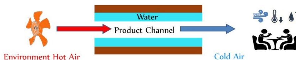
The Direct Evaporative Cooling System
