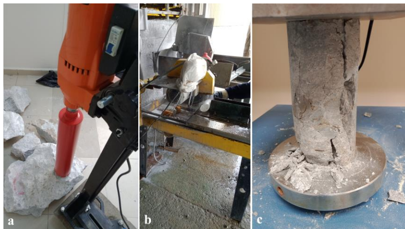
Figure 2. a) Rock specimen coring, b) core cutting, c) uniaxial compressive strength testing
