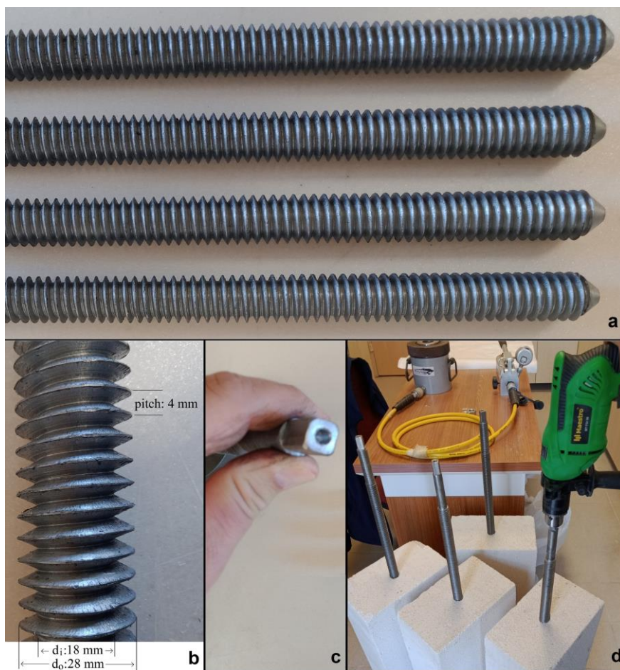
Figure 5. a) and b) thread designs of laboratory specimens, c) a shown of the square-shaped end of the screw bolts, d) a photo of screw bolt insertion in the laboratory study
