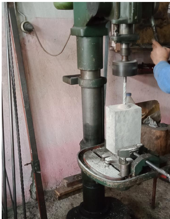
Figure 4. Rock block drilling
