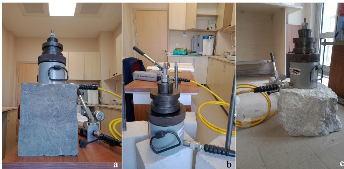
Figure 8. Some photos from pull-out tests of screw bolt specimens used in the laboratory study
