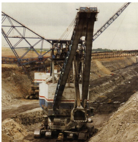
Fig. 2a Tandem operation of a cross-pit BWE and a stripping shovel [5].
