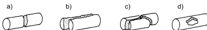
Figure 3. According to ISRM (a-c) valid test, (d) invalid test for the diametrically loaded body [4]
