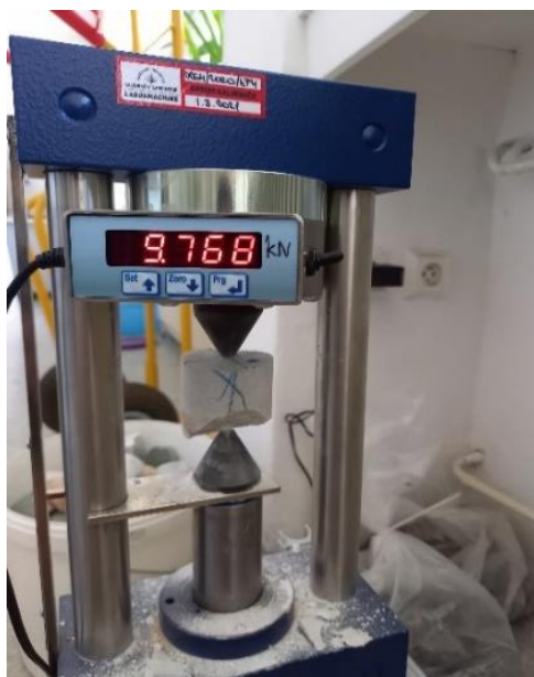
Figure 1. Point Load test (photo by ŠANCER,2022)
