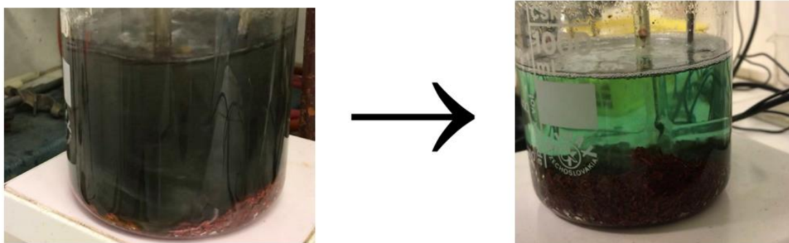
Figure 2. Discoloration of the sample after 15 minutes of cementation
