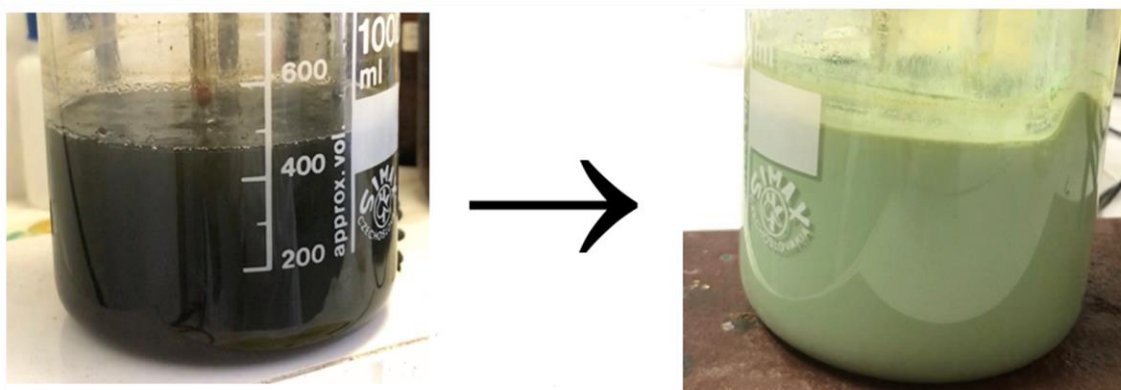
Figure 4. Change of colour and consistency of the solution during the precipitation process
