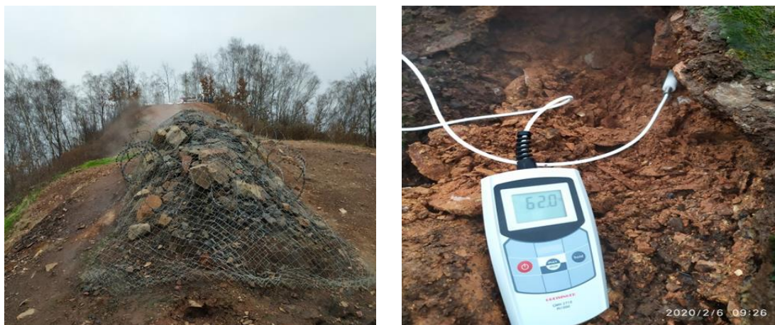
Figure 1. Manifestations of thermal activity on the Ema dump (left), measured temperature at the sampling point (right) [Kuřová, 2020]
