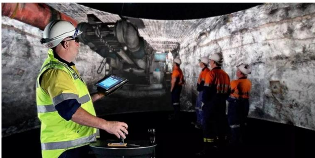
Figure 1. VR simulator CAVE system [8]
