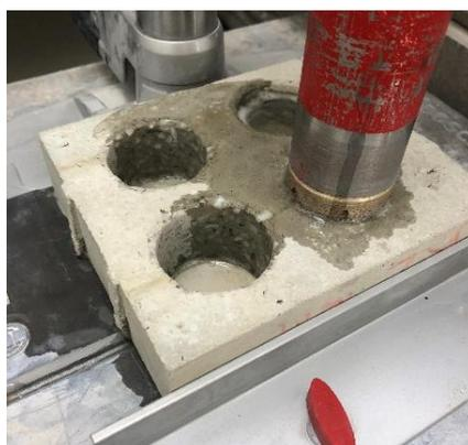
*Figure 1. Test specimens preparation process*
