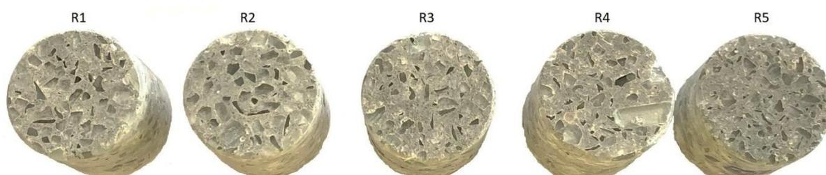
*Figure 2. Structure of the test specimens prepared according to formulas R1 to R5*
