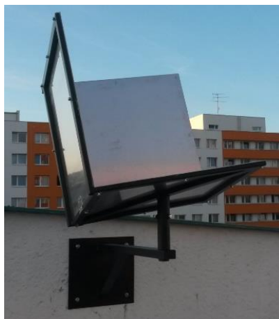
Figure 2. Used construction of corner reflector CR1
