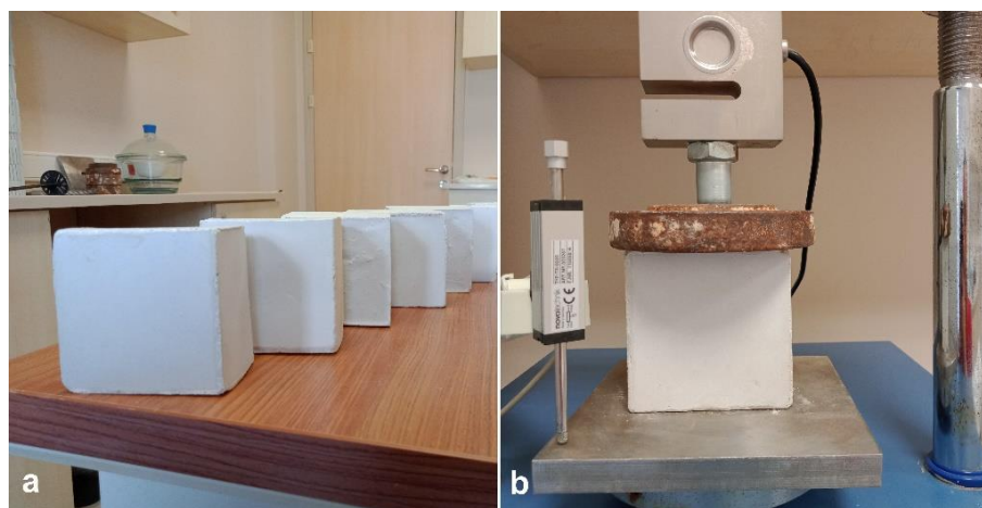
Figure 5. a) FC samples, b) UCS test of FC samples
