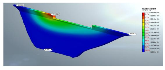
Figure 14. Displacement at the end of the second earthquake
