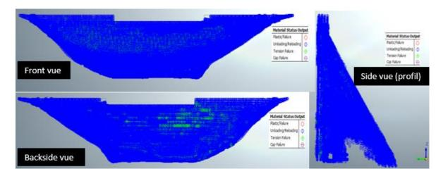
Figure 15. Plasticity state of the first earthquake
