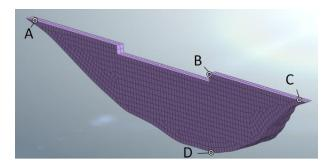
Figure 6. Reference points for the behaviour dam analysis
