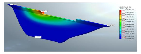
Figure 13. Displacement at the end of the first earthquake
