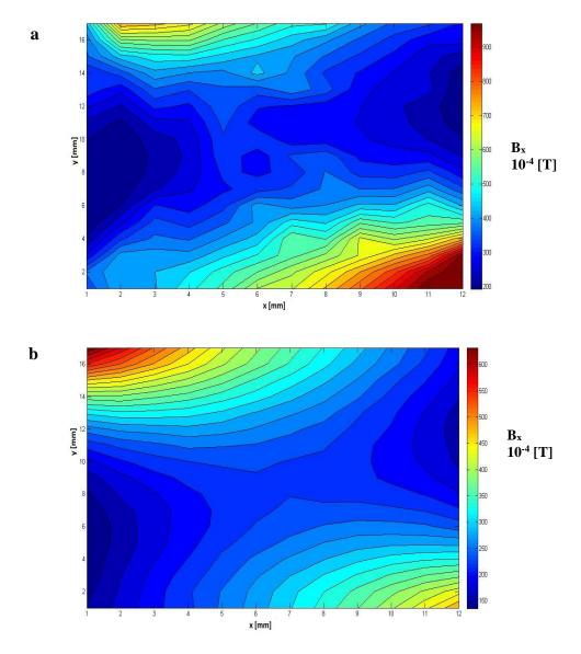
Fig. 4 Distribution of  $B_x$  in the measured sample area: (a) before annealing, (b) after annealing. (I1==0.11A, U1=0.9V vertical coil; I2= -0.9A, U2=-0.8V horizontal coils), (z = 3 mm).GeoScience EngineeringVolume LX (2014), No.2http://gse.vsb.czp. 1-7, ISSN 1802-5420
