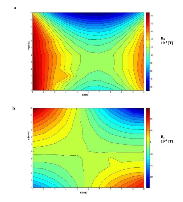
Fig. 5 (a) The  $B_x$  component of magnetic induction in detail in the measured area in a depth z = 3mm at 2.5 A current in coils, the measure detector is horizontal; (b) the  $B_y$  component of magnetic induction in detail in the measured area in a depth z = 3mm at 2.5 A current in coils, the measure detector is horizontal.
