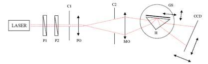
Fig. 1 Measuring apparatus for Dark Mode Spectroscopy. P1, P2 – polarizers, C1; C2 - shutters, FO - lens, MO - microscope objective lens, H – coupling prism, GS - rotation table, CCD camera.
