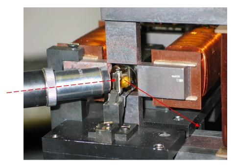
Fig. 3 Detail of pole extensions of magnetic field source for DMS.
