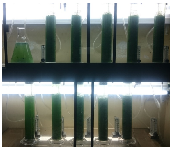
Photo 2.2: Array of glass cylinders to grow microalga spirulina with injection of commercial and HEVA \text{CO}_2 .
