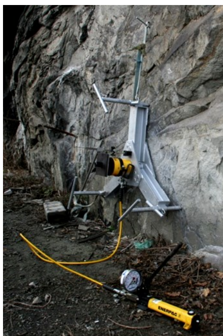
Fig. 1 Loading stand with hydraulic system
